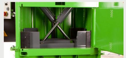
Cross ram and long-stroke cylinder for optimum compression in a small space
