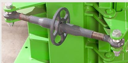
Integrated kicker for easy bale removal, bales tied with two rolls of string and heavy duty door clamp
