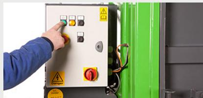
Automatic and manual cycles for cardboard versus higher-memory material like plastic
